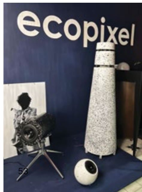
ALTO - Free standing, with down-facing bass reflex, active class D amplified Bluetooth speaker unit.
